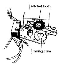
**3.** Turn the timing cam by hand until the "V"-shaped notch lines up below the ratchet tooth.
